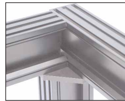
Loads bearing on the top rails are supported directly on the legs, unlike other systems that rely on fastener friction in T-slots for support.
