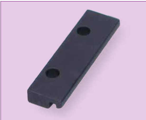
Four BiSlide cleats are available: standard one- and two-hole, sandwich, and an optical cleat. Pictured is the standard cleat used to mount a BiSlide to a base, frame or to another BiSlide Assembly. Each pair has 425 lbs. of holding capability.
