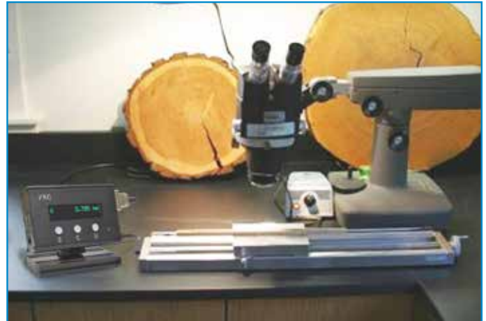
Although used in Dendrochronology, the Velmex TA System has been used in the study of mollusks, probe positioning, bore camera inspection, material stress analysis and other research.
